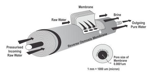
Reverse Osmosis is aprocess in which water is forced through a semi-permeable membrane by applying very strong pressure. Therefore only fine water molecules can pass through the membrane. All contaminants such as bacteria, viruses, herbicide, heavy metals and chemical poisons are removed. With added special features, the actual container and dirty water with impurities is discharged.
